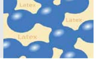
The mold is vulcanized at 115° Celsius; the cells continue to expand, giving the material its elastic properties. This latex core is further worked upon to create the high quality THOMSEN mattresses, pillows, and toppers.
