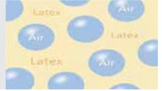
The mixture is flash frozen to -30° Celsius, enabling the cells to retain their round form. The cell membranes break open and link together to create an open-cell structure.
